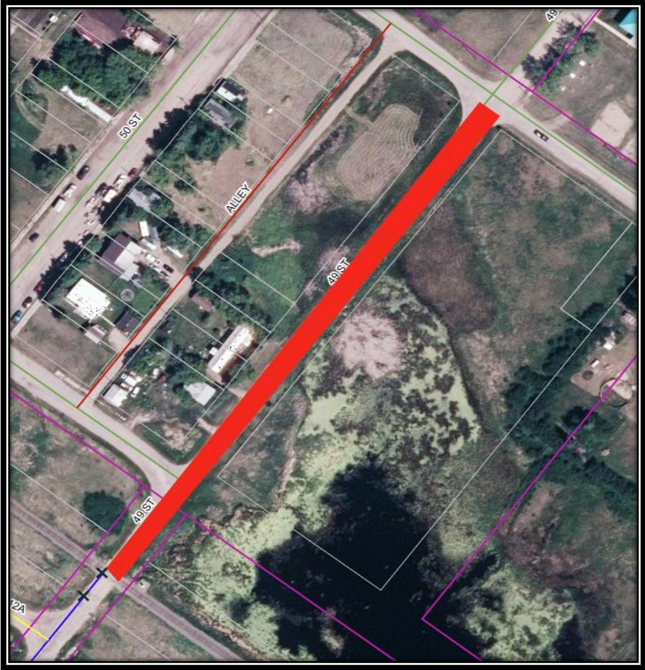
240M – Re-oiling of rutting, potholes and rough patching
