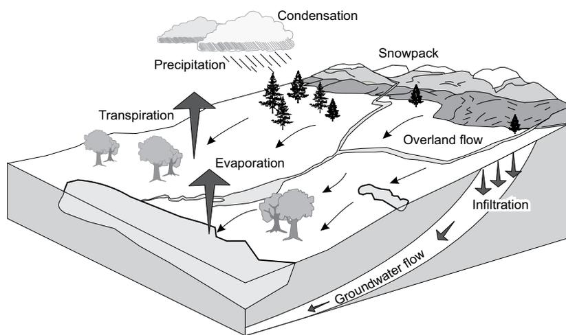
Some precipitation that falls to the ground surface infiltrates the ground and becomes groundwater. Groundwater is defined as sub-surface water that fills openings and pore spaces in soil and rock layers. Below the ground surface is an unsaturated zone, which water travels through, to reach lower zones. The water table is the point at which the ground is completely saturated. Below this level the pore spaces between every grain of soil and rock crevice completely fill with water.
